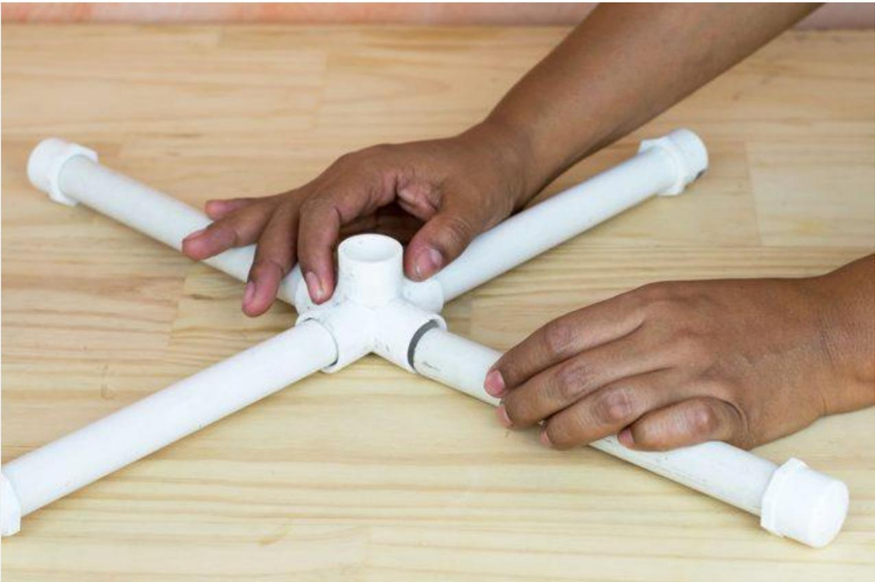
Insert four 2-foot PVC pipes into a five-way cross connector so that they form a foot for the pole. Slide an end cap on each pipe.
