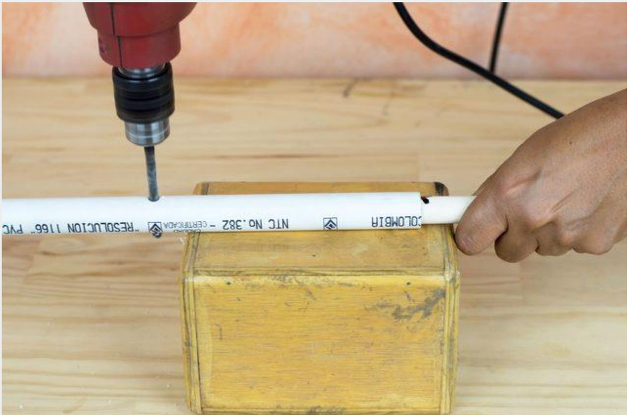
Slide the smaller pole inside the larger one. Line up the first X on the smaller pipe with the hole you drilled in the larger one. Holding it firmly, drill through the smaller pipe while it is inside the larger one. The drilled holes should line up and allow you to insert the ringed pin all the way through both pipes.
