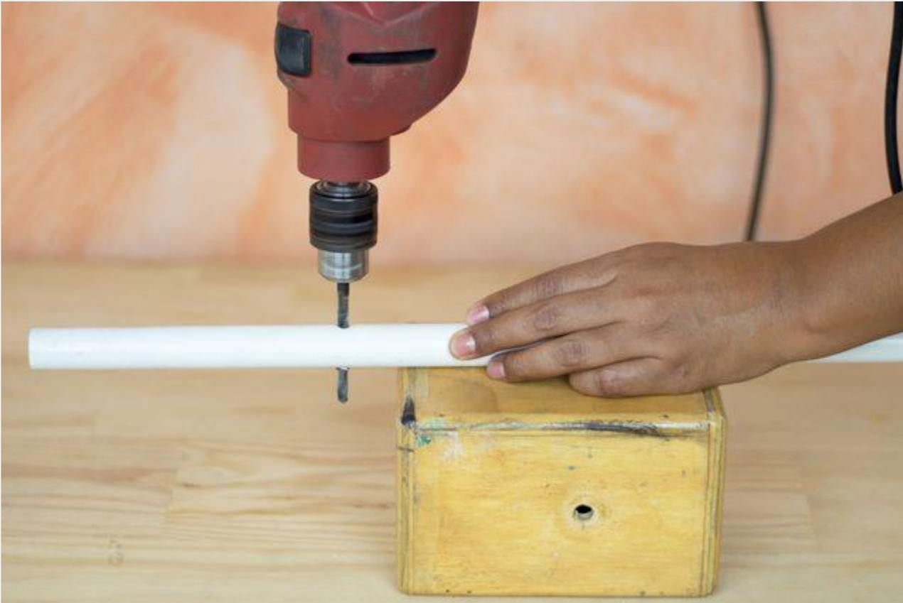
Drill a hole through the middle of the pipe, making another hole on the opposite side. Be careful to make the holes even. They should be equal distances from the top and bisect the pole through the middle. Make the hole slightly larger than the ringed pin.
